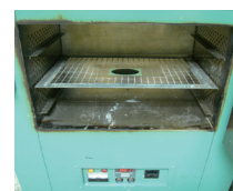
A.2 Store the specimen in the oven at 80°C for an hour. Then, take it out.
