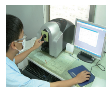
A.4 Measure delta E, and compare it with its delta E value measured prior to the testing.
