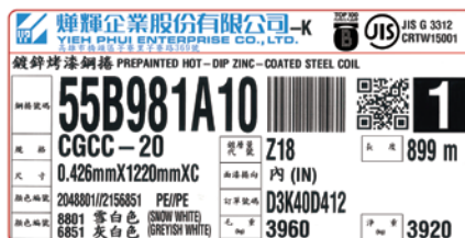
焊辉烤漆产品之标签示范 Yieh Phui sample of product ID label for prepainted metallic coated steel coil
