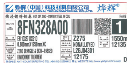
焊辉(中国)镀锌产品之标签范例 Yieh Phui (China) sample of product ID label for metallic coated steel coil
