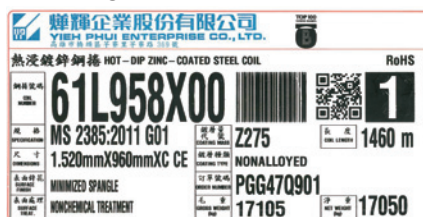
焊辉镀锌产品之标签示范 Yieh Phui sample of product ID label for metallic coated steel coil
